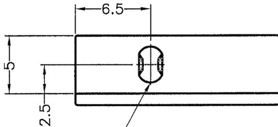
MOUNTING HOLE  $\phi$ 2.5mm
