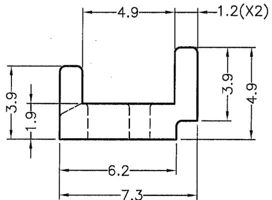
NOTE:1. All measurement does not include gate which raises under 0.3mm.
