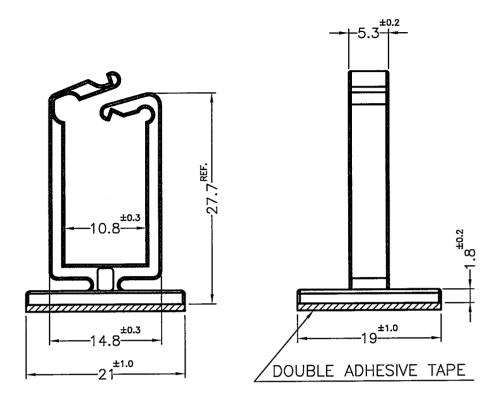
NOTE:1. THE PRODUCT SIZE IS NOT INCLUDED THE SIZES OF ADHESIVE TAPE AND ITS LINER. 產品尺寸皆不含背膠及離型紙.
