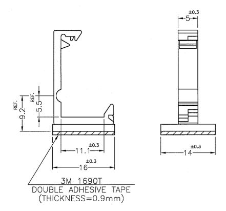
NOTE:1. THE PRODUCT SIZE IS NOT INCLUDED THE SIZES OF ADHESIVE TAPE AND ITS LINER. 產品尺寸皆不含背膠及離型紙.
