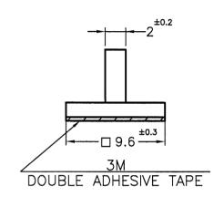
NOTE: 1. HEIGHT INCLUDE ADHESIVE TAPE, NOT INCLUDE RELEASE PAPER.
