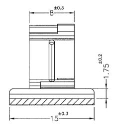
NOTE:1. THE PRODUCT SIZE IS NOT INCLUDED THE SIZES OF ADHESIVE TAPE AND ITS LINER. 產品尺寸皆不含背膠及離型紙.
