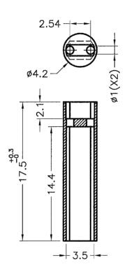
NOTE: All measurement does not include gate which raises under 0.3mm.
