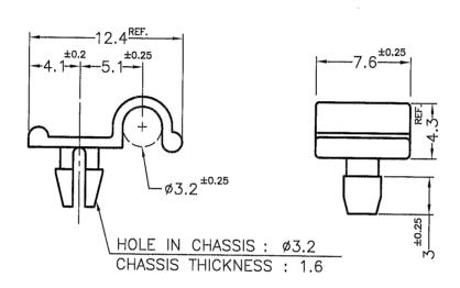
NOTE:1. All measurement does not include gate which raises under 0.3mm. 2. It is normal if it is shrinking.
